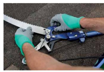
A saw blade is included for any larger branches that are too big to fit between the jaws of the pruner.
